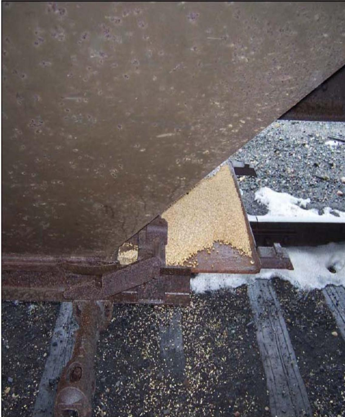
EXHIBIT - H / Grain Hopper Car Allowed to Move with Gate Open. Grain has vibrated to bottom of chute, and is released to ground as do other substances such as potash and other powdered chemicals.
