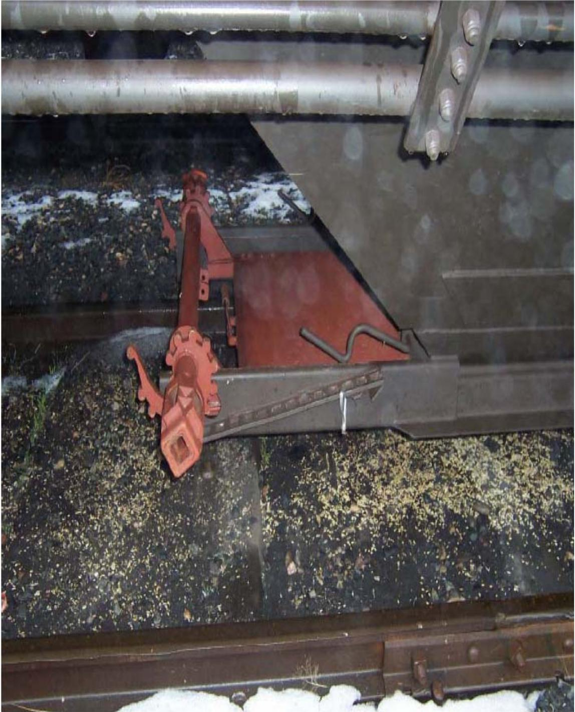
EXHIBIT - I / Grain Hopper Car With Gate Left Fully Open at Extreme End Of Gate Guides.
