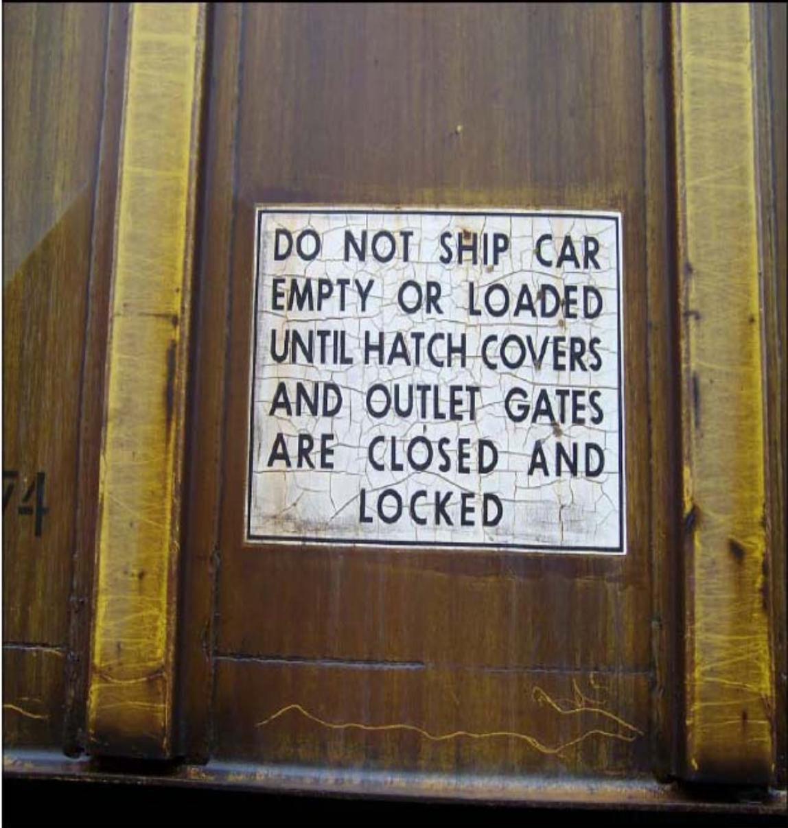
EXHIBIT - J / Signage on Sides of Cars Indicating To Ship Car With Outlet Gates Closed and Locked.
