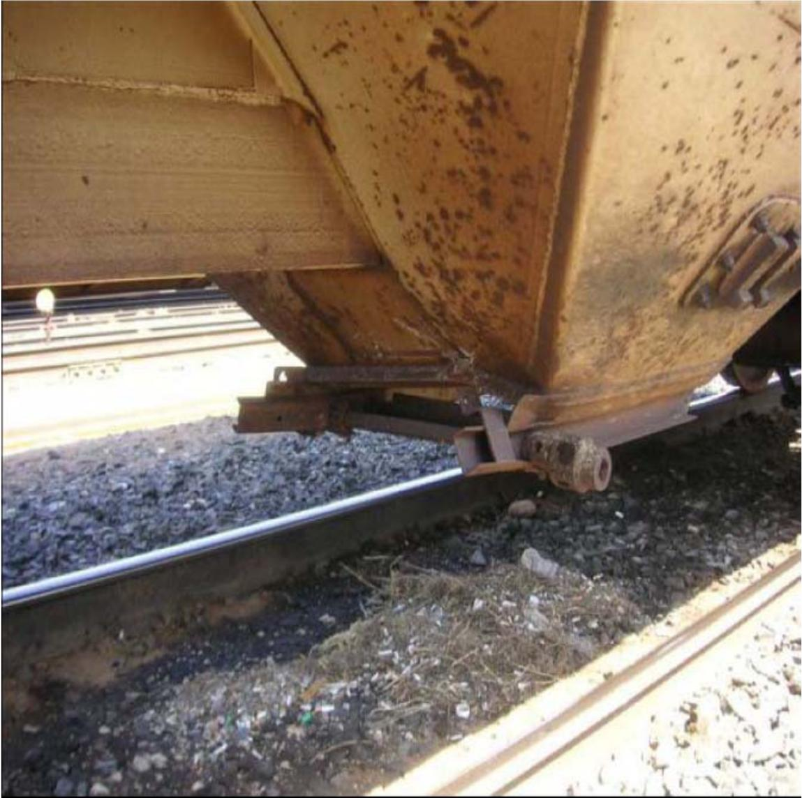
EXHIBIT - G / Damage to Hopper Car Resulting After Gate Dislodged While in Transit
